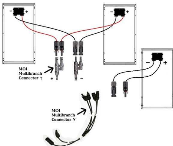
Fig. 7.3.3 Connection of PV moudles using MC4 connectors
