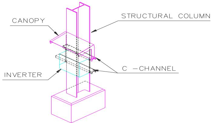
Fig. 7.4.4 Support structure for installation of inverter
