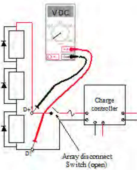
Fig. 10.2.5 Measuring the open circuit voltage of array
