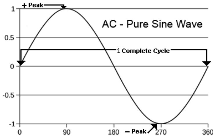
Fig 2.2.4 AC waveform – Single Phase Supply
