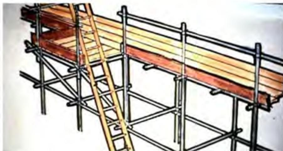
Fig. 11.4.5 Guardrails
