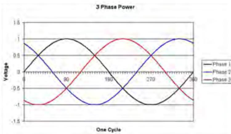
Fig 2.2.6 AC Waveform – Three Phase Supply
