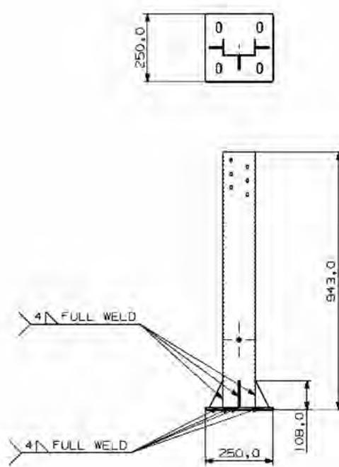
Fig. 7.1.6 Sample design for installing mounting post
