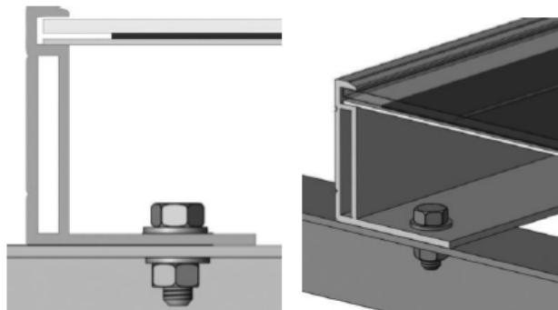
Fig. 7.3.1 Module mounting by using bolts
