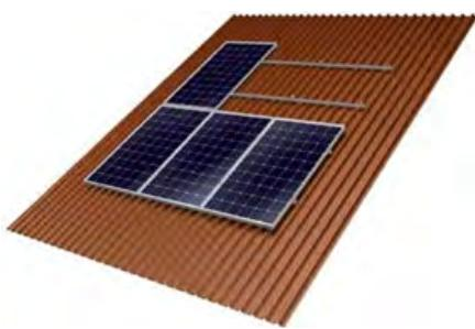
4. **Rails and racks** This is a flexible system for the parallel mounting of framed and unframed modules on all current types of trapezoidal metal sheet roofs. Fast and easy mounting is guaranteed due to the unique hook design of its fasteners. These fasteners are easily fixed to the side of the standing seam. The lateral position of the screws in the profiled sheet has a positive effect on the permitted tearing levels. It allows for easy adjustment and levelling of minor height deflections
