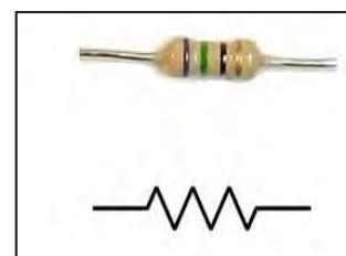
Fig 2.2.12 Resistor (with symbol)
