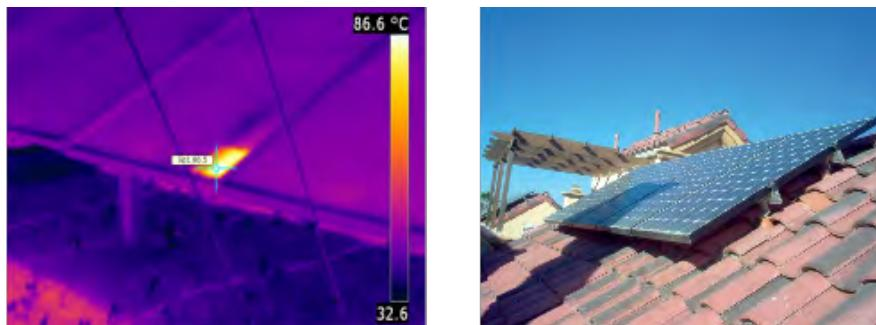
Fig. 9.3.1 Spot shading causes hot spot and may damage a module
