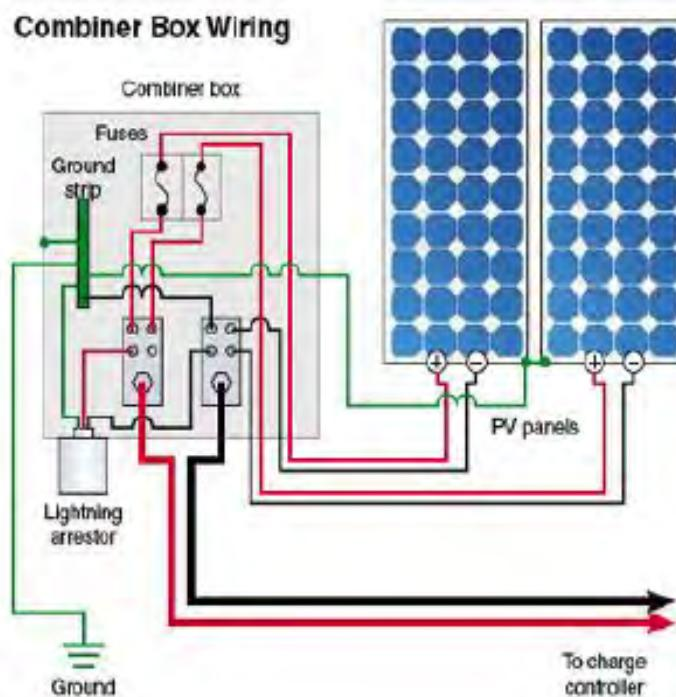
Fig. 7.3.5 Schematic diagram of grounding Solar PV Panels
