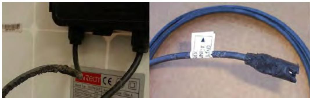
Fig. 10.2.15 Physically damaged wires
