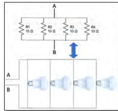
Fig. 2.3.2 Parallel connected LED lamps
