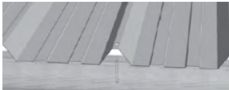
**STEP 2:** Screw in hanger bolt
