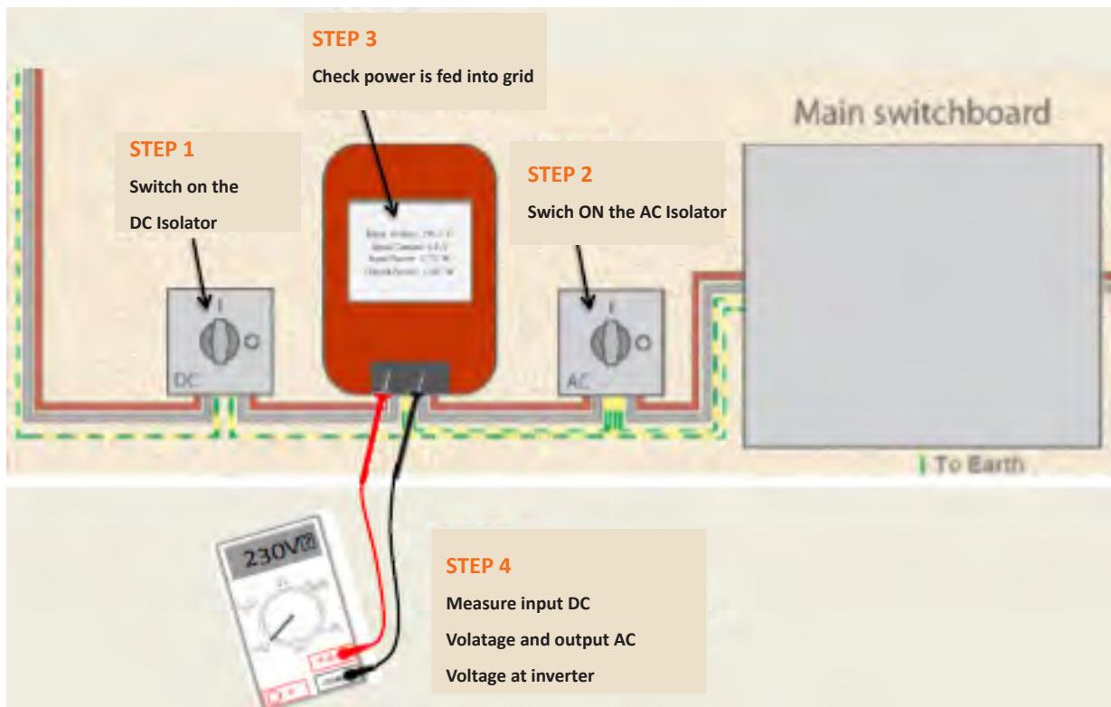
Fig. 9.7.2 Start up of grid connected inverter
