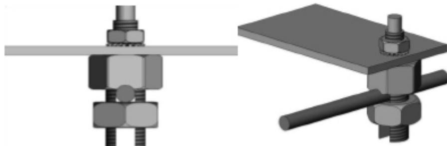
Fig. 7.3.4 Grounding of modules using earth ground electrode
