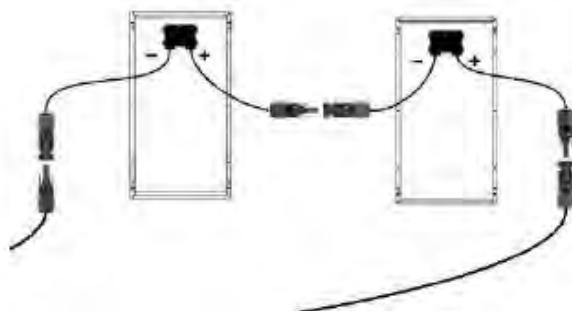
Fig. 8.3.2 Diagram for connection of PV modules
