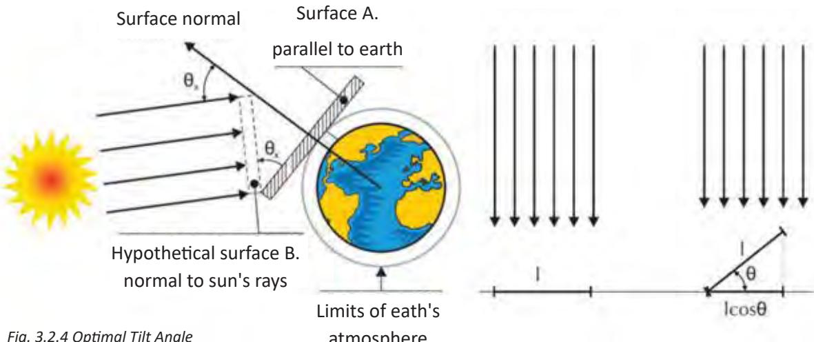
Fig. 3.2.4 Optimal Tilt Angle
