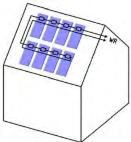
**Method 2***Fig. 2.6.1 The module cables should be placed close together (Method 2)*
