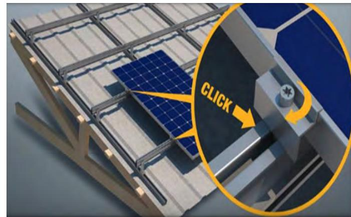
**STEP 6:** Now fix the PV modules & Level it over elevated structure
