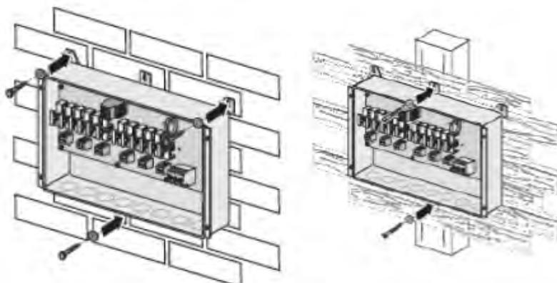
Fig. 8.2.1 Wall & structure mounting of DC Combiner Box
