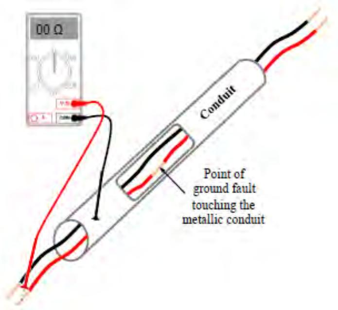
Fig. 10.2.17 Finding a ground fault
