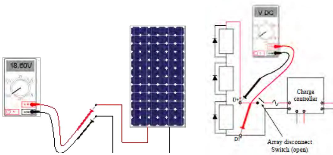
Fig. 9.3.4 Measuring module and string open circuit voltage
