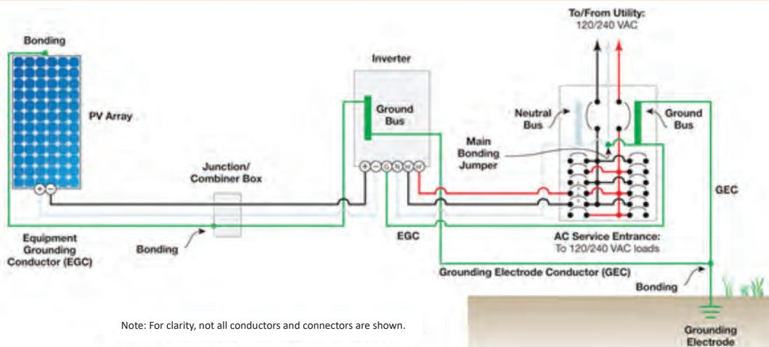
Fig. 2.6.4 Earthing/Grounding of a Solar PV System
