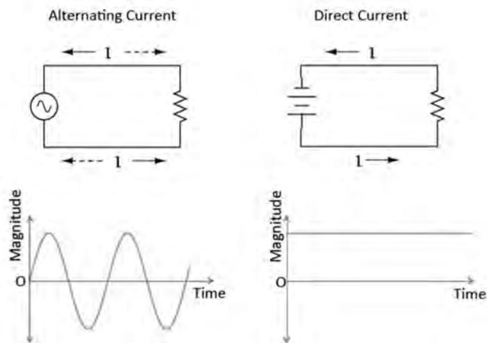
Fig 2.2.2 Alternating Current and Direct Current - Circuit and Waveforms
