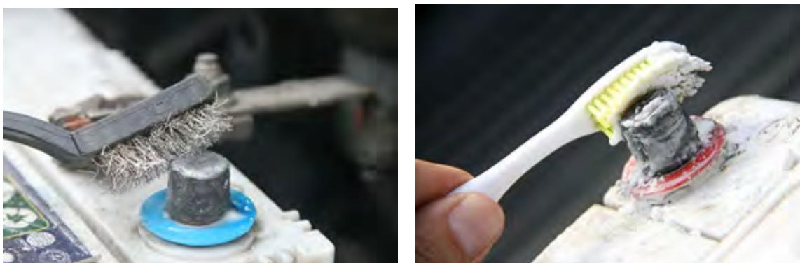
Fig. 10.2.11 Cleaning of batteries terminals to avoid corrosion and loose connections
