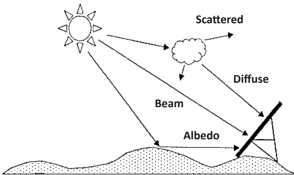
Fig. 3.1.2 Global horizontal radiance is the sum total of all radiation (beam, diffuse and albedo) falling on the solar pv panel
