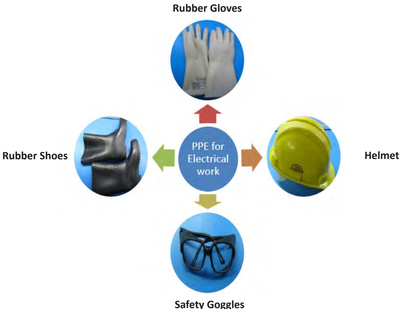
Fig. 8.1.2 Personal Protective Equipment (PPE) for Electrical Work
