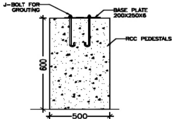
Fig. 7.1.4 Side view of an RCC pedestal
