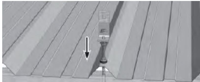
**STEP 5:** Install module support/racking frame
