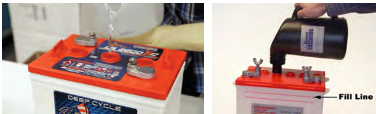
Fig. 10.2.10 Top up of batteries
