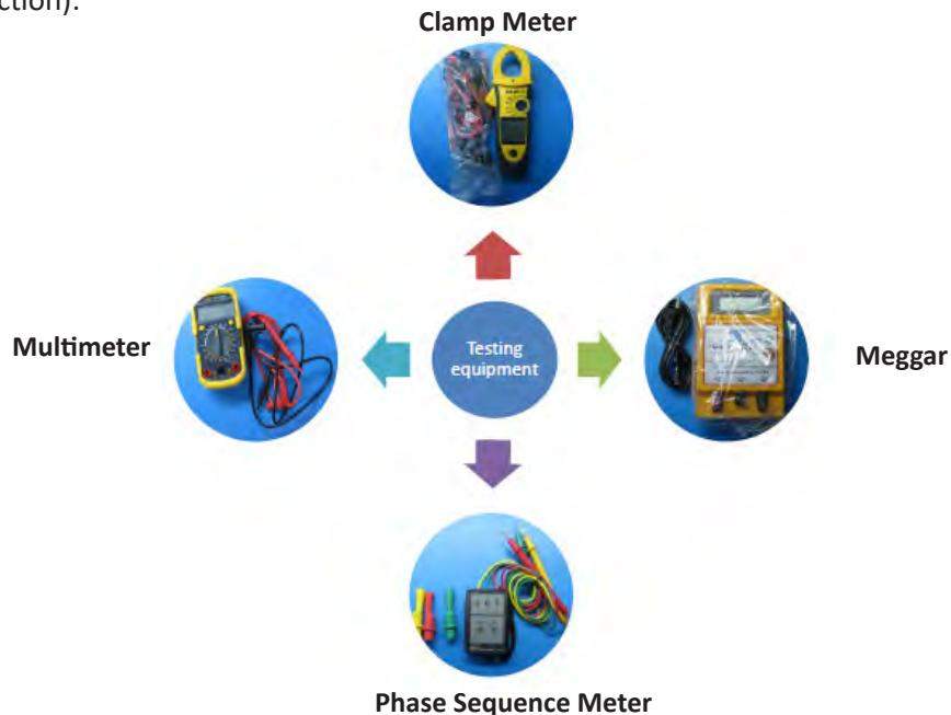
Fig. 8.1.4 Testing equipment
