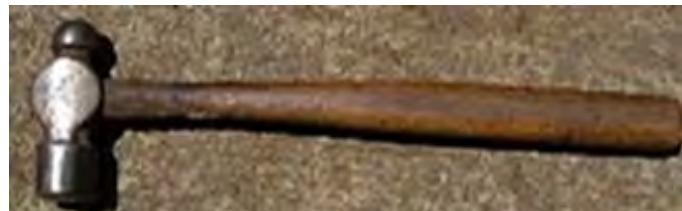
**Uses:** Though the process of peening (surface hardening by impact) has become rarer in metal fabrication, the ball-peen hammer remains useful for many tasks, such as striking punches and chisels (usually performed with the flat face of the hammer). The peening face is useful for rounding off edges of metal pins and fasteners, such as rivets.
