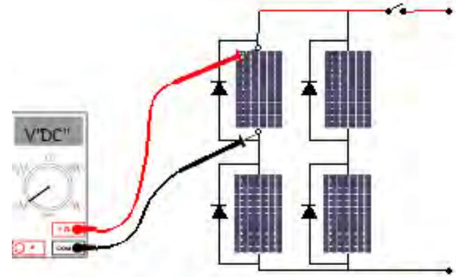
Fig. 10.2.6 Measuring the open circuit voltage of module
