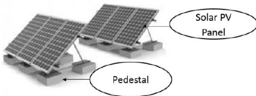
Fig. 7.1.1 Pedestal type of footing
