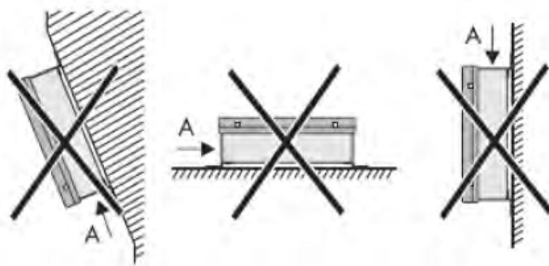
Fig. 8.2.2 Wrong mounting of DC Combiner Box (SMA)
