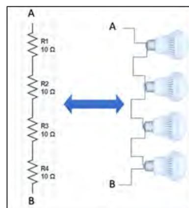
Fig. 2.3.1 Series connected LED lamps
