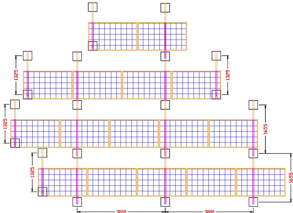
Fig. 7.2.3 Plan view of the PV system arrangement
