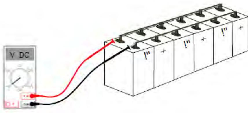
Fig. 10.2.12 Battery load tests using a multimeter (Voltmeter)
