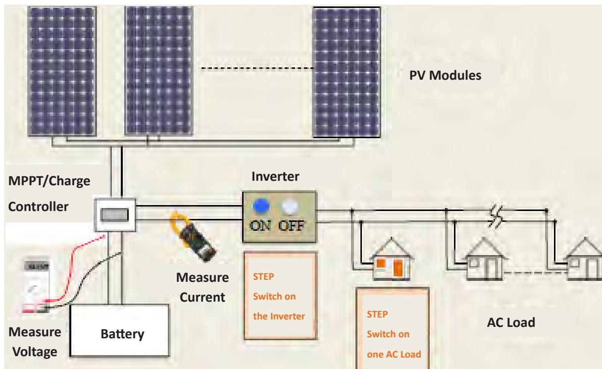
Fig. 9.7.1 Start up of standalone PV system
