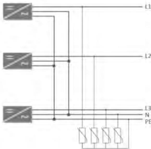
Fig. 2.6.3 Surge protection device (SPD) is connected between the junction box and inverter
