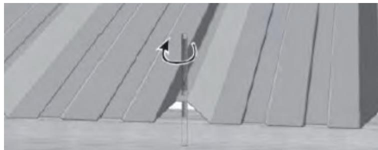
**STEP 3:** Place rubber seal and spacer, screw nut on and tighten
