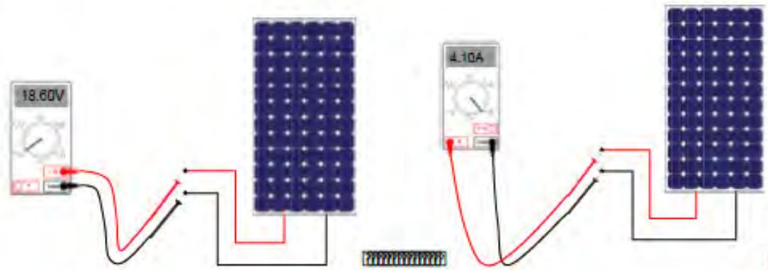
Fig. 10.2.4 Checking current and voltage of PV modules
