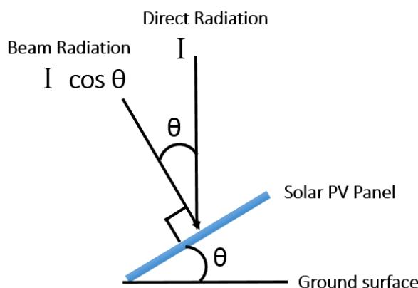
Fig. 3.1.1 cosine component of direct radiation is called
