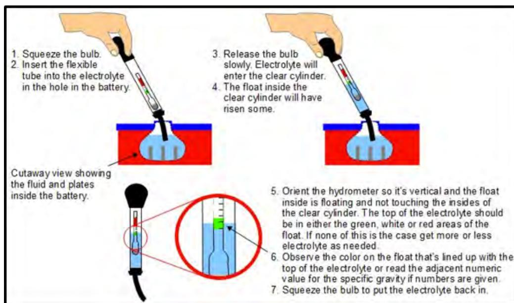
Fig. 10.2.9 Maintenance of battery by testing the electrolyte
